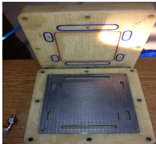
Figure 7. Test fixture for bipolar plate leakage test
