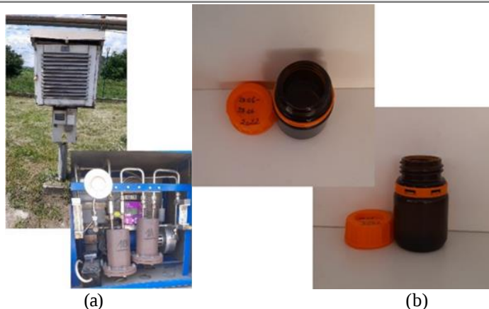
Figure 3. Air sampling station (a) and the open vial used for laboratory atmosphere monitoring (b)
