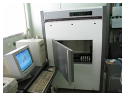
Figure 4. Ultra-Low Level Liquid Scintillation Spectrometers 1220 QUANTULUS
