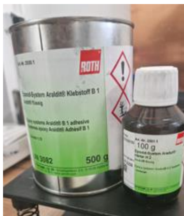
Figure 6. Araldite and curing agent procured from ROTH used for sample SCP3/4.
