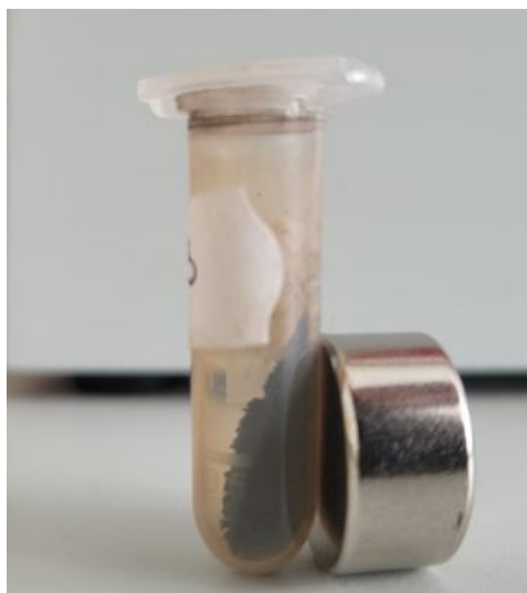
Figure 1. Powder of magnetite attracted by the magnet
